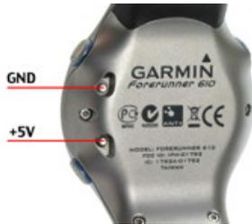
In case you decide to make your own power connector, you can see the pinout in the picture above. Please notice though that the rear of the watch is made of metal and hence conducting electricity, so making a connector without risking a short circuit might prove a little difficult. It's probably better to buy an extra cable at eBay <sup>[5]</sup>.
